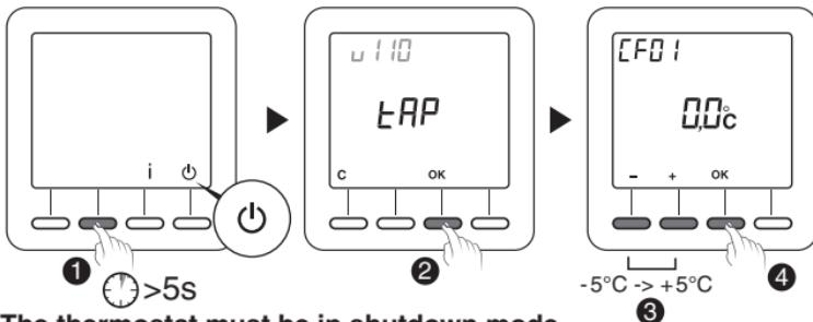
**The thermostat must be in shutdown mode.**
