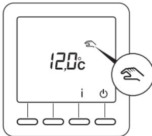
During the external override, if the symbol
